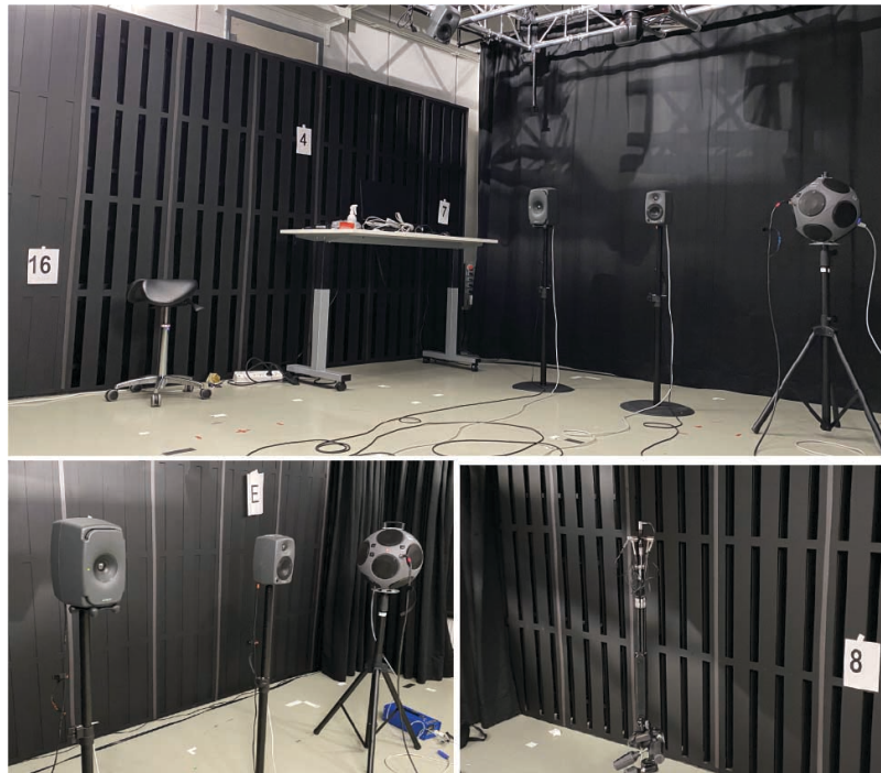
Figure 2 Measurement devices, Genelec 8331A, Genelec 8020B and Omnidirectional loudspeaker 01dB LS01. The microphone array has six omnidirectional capsules.
