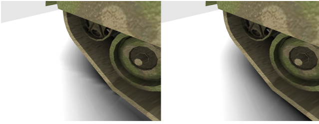
Figure 5: Left: Artifacts caused by undersampling. Right: The result achieved by downsampling from a higher resolution with a Gaussian reconstruction filter. Both images are using the same 32 \times 32 resolution for the cube maps. Contrast has been adjusted to highlight the artifact.
