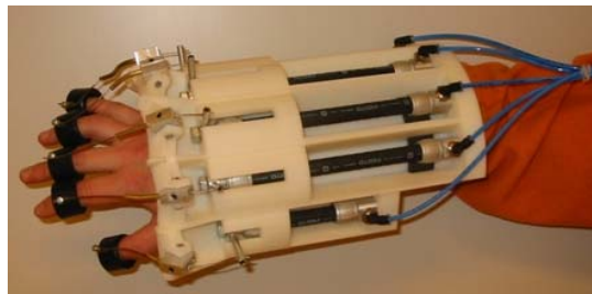
Figure 2. First prototype of haptic glove with McKibben muscles.
