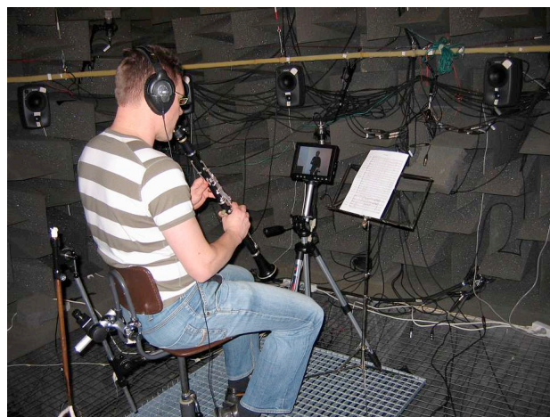
Figure 1. The recording configuration in an anechoic chamber. A musician followed the conductor through the monitor and listened to the piano version of the whole score while playing his/her own part.
