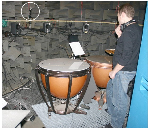
Figure 3. Positioning of the timpani in anechoic chamber. Microphone no. 6 in forward direction is circled.
